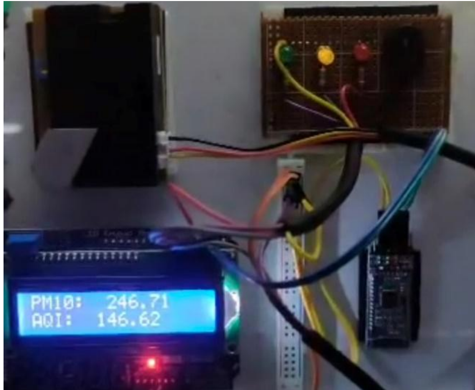
Fig.7.Experimental AQI data is displayed in real-time on the LCD.
