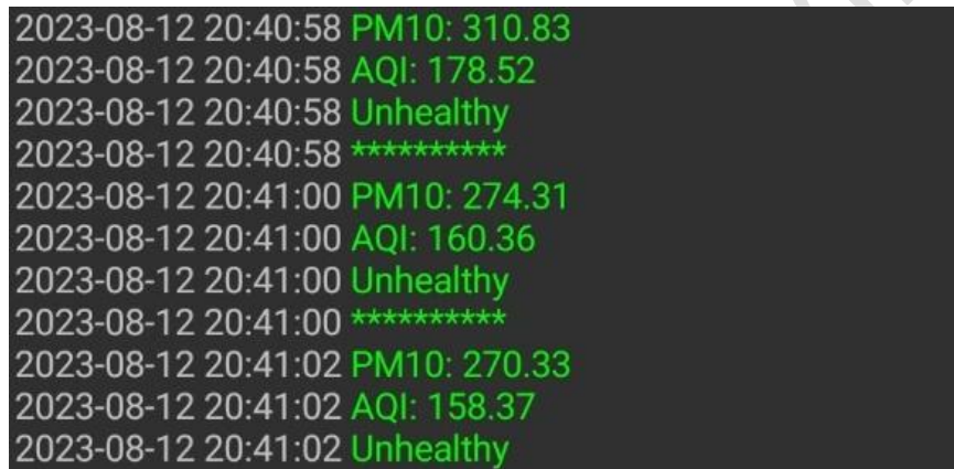
Fig.10. Experimental AQI data is displayed in real-time on the Bluetooth-connected device.
