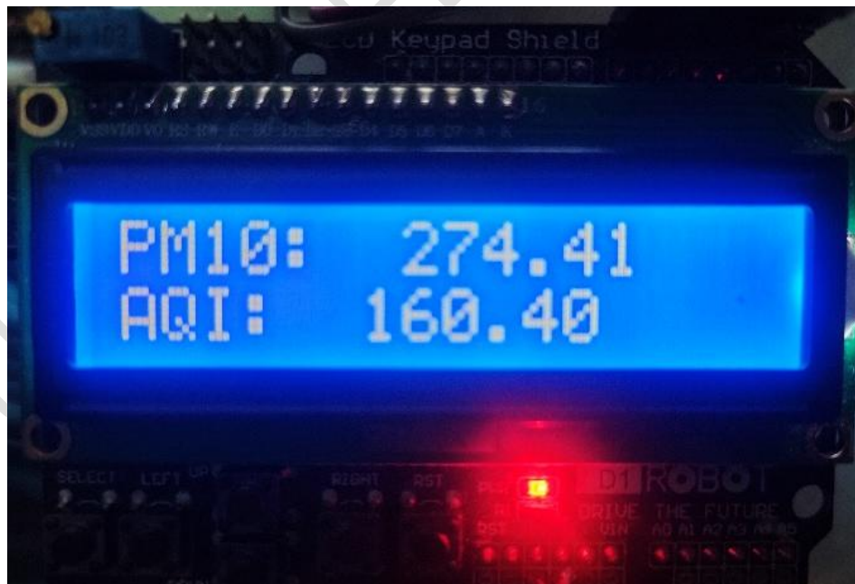
Fig.8.Experimental AQI data is displayed in real-time on the LCD with a red LED indicator.
