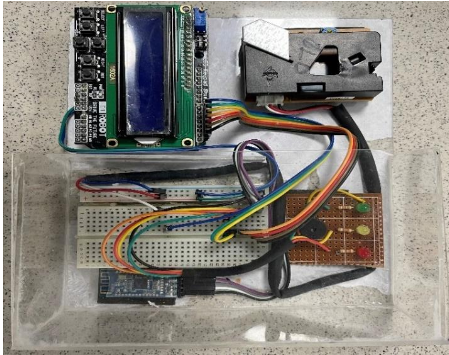
Fig.6.Portable air quality detector using Arduino with acrylic cover.
