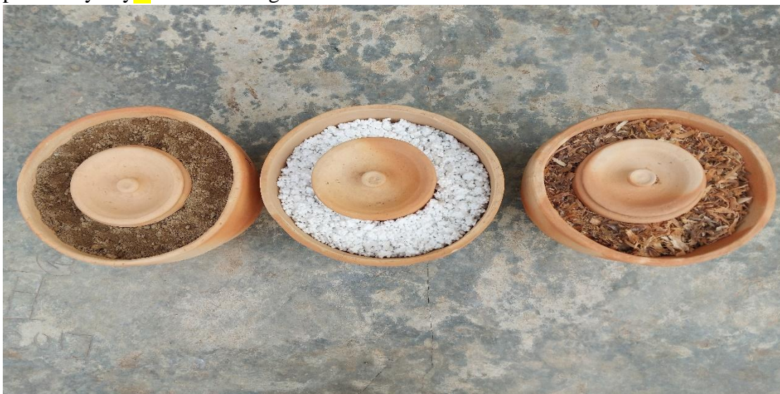
Figure 3. Zeer pot refrigerators with different lining media
