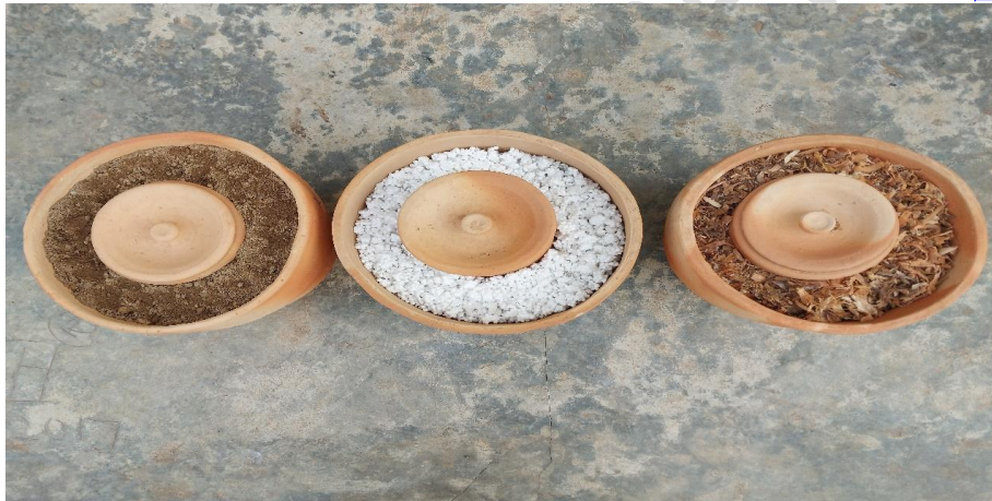
Figure 3. Zeer pot refrigerators with different lining media
