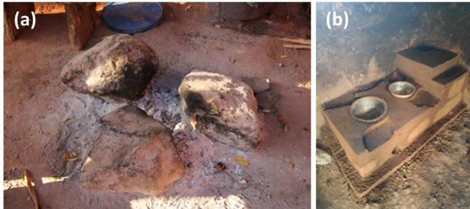
Figure 1. Types of stoves (a) Three-Stone Fire stove and (b) mud stove (Donegan, 2018)
