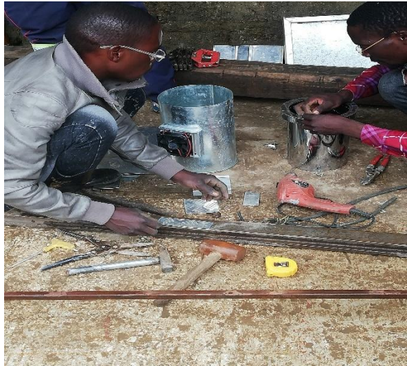
Figure 7. Fabrication of outer casing and combustion chamber.
