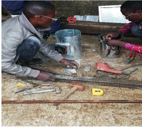
Figure 7. Fabrication of outer casing and combustion chamber.
