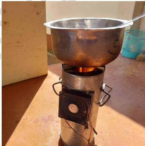
Figure 8. TEG testing on the ICS.
