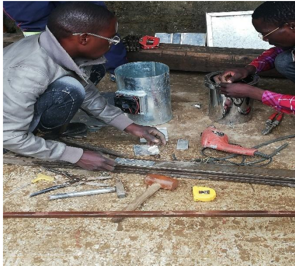
Figure 7. Fabrication of outer casing and combustion chamber.
