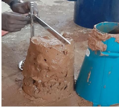
Figure 1. Slump of fresh geopolymer concrete mix
