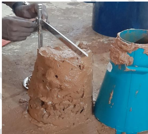
Figure 1. Slump of fresh geopolymer concrete mix
