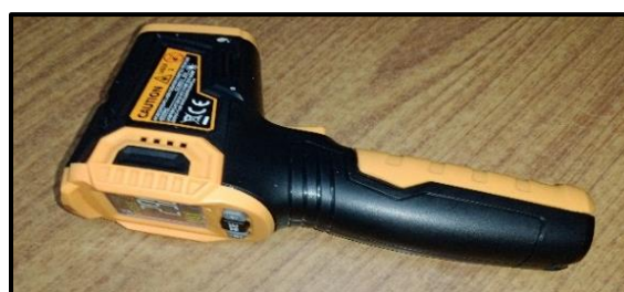
Fig .3 Portable Infra-red Thermometer
