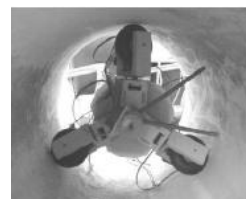
(B) Pipeline scale cleaning and detection robot
