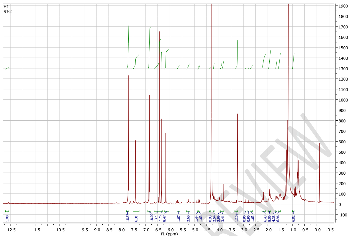
Figure 4: The 1 H-NMR Spectrum of Apigenin (4', 5, 7-trihydroxyflavone)
