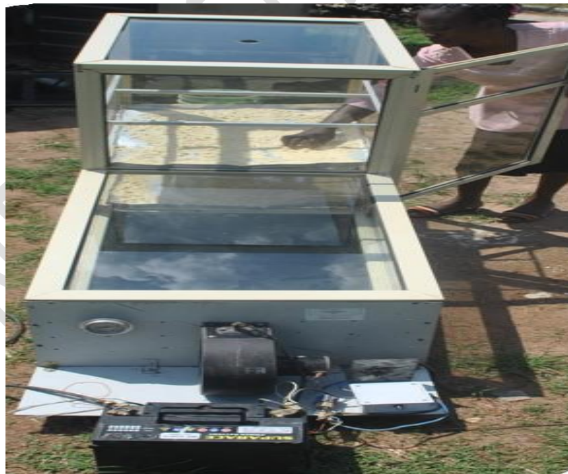
Fig. 2. Experimental set-up showing cassava grates drying process.
