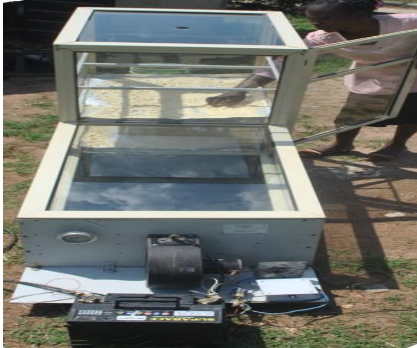
Figure 2: Experimental set-up showing cassava grates drying process.
