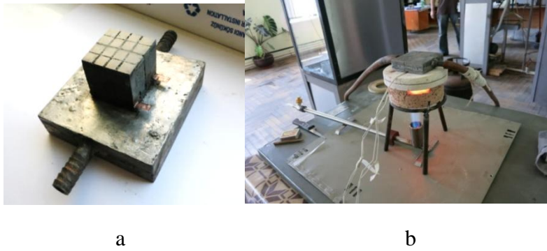
Fig. 7. a - thermoelectric module connected to water cooler, b - thermoelectric module testing.
