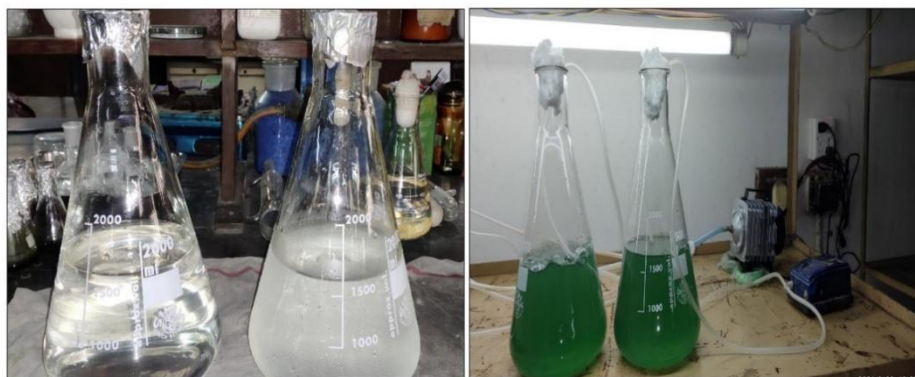
Fig. 1. (a): Zarrouk medium without NaHCO 3 (b) Extracting Supernatant added to the medium after autoclaving.
