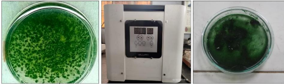
Fig.5. Recovery of biomass by Centrifuge
