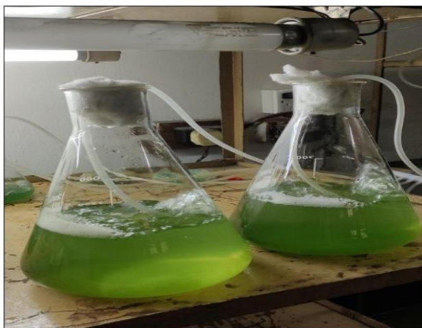
Fig. 3. CO 2 absorbent NaOH added to specific one flask and the other controls.
