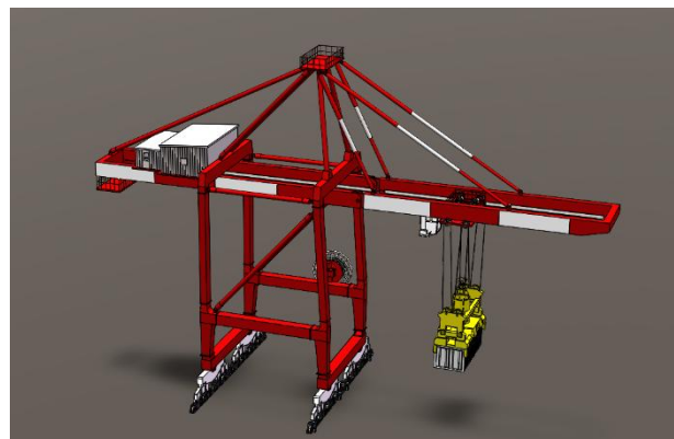
Figure 8. Geometric model of container crane on shore
