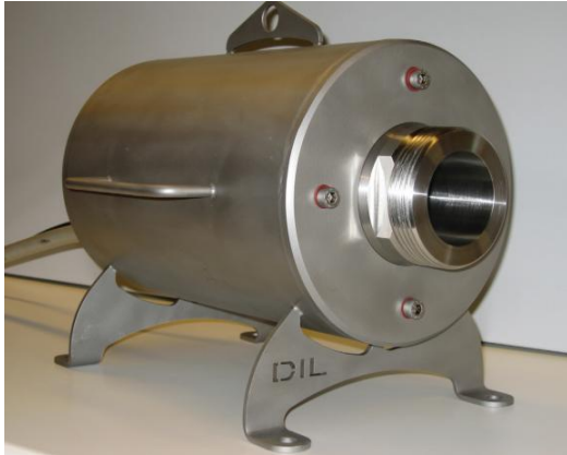
Figure 2.: A continuous flow PEF treatment chamber with a diameter of 60 mm[12].
