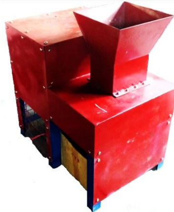
Fig. 3. Fabricated PET bottle shredding machine
