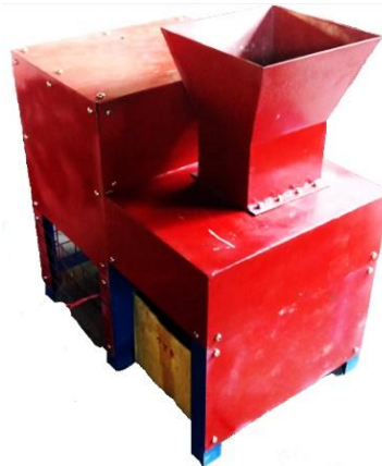
Fig. 3. Fabricated PET bottle shredding machine
