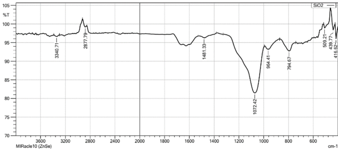
Fig. 1 FTIR spectrum of Mesoporous Nano Silica (MNS)
