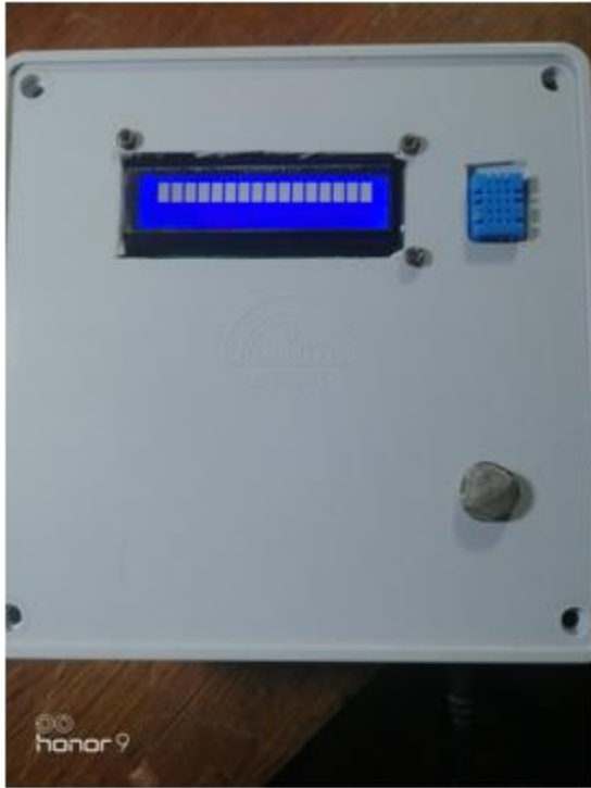
Fig.7.Initialization Screen of air quality monitoring system
