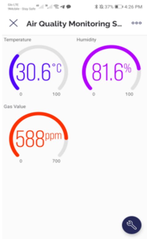
Fig. 11. Data of temperature, relative humidity an air quality on mobile app
