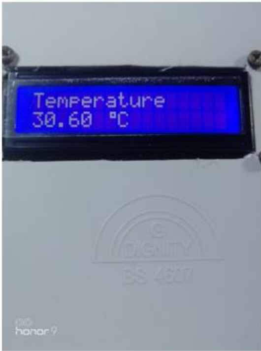
Fig. 8.Data of Temperature on LCD Screen Fig. 9. Data of relative humidity on LCD Screen
