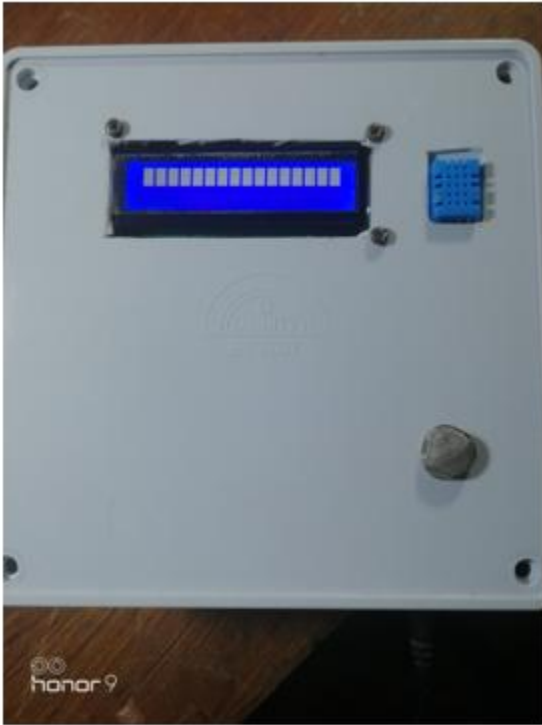
Fig 7 Initialization Screen of air quality monitoring system
