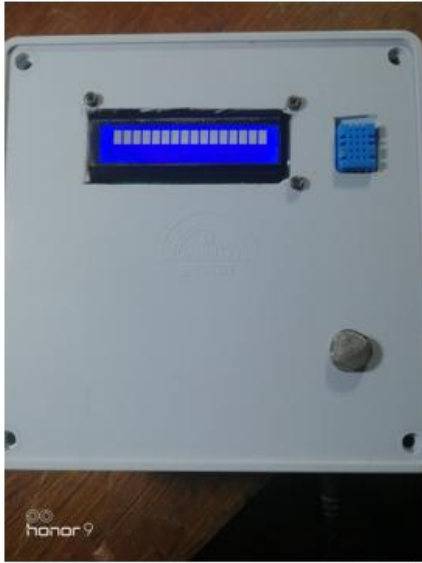
Fig.7. Initialization Screen of air quality monitoring system
