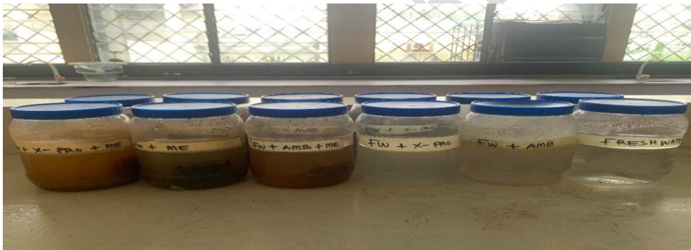
Plate 1: effluent preparation of toxicants (metals with corrosion inhibitors soaked in fresh and brackish water for 30 days before toxicity setup)
