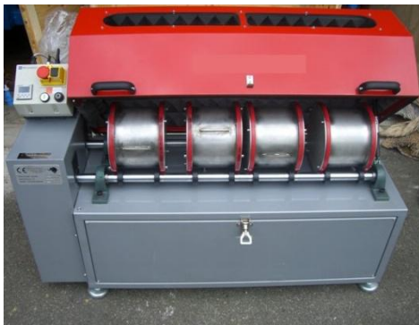
Figure 4: Micro Deval Test Match
