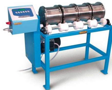
Figure 4: Micro Deval Test Match
