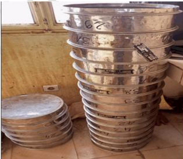
Figure 1: Series of sieves for particle size analysis. Source: University of Technology and Management laboratory.
