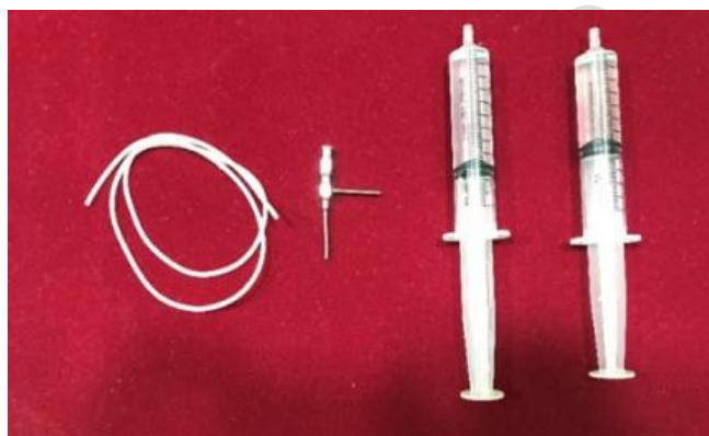
Fig. 1. Co-axial method of electrospinning
