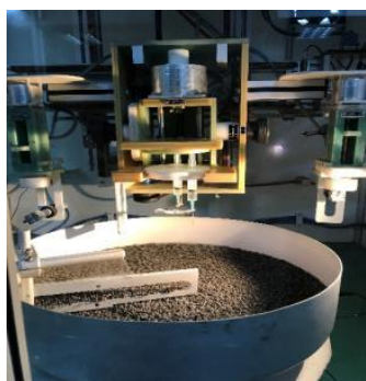
Fig. 2. Vertical electrospinning unit for coating seeds with fibre
