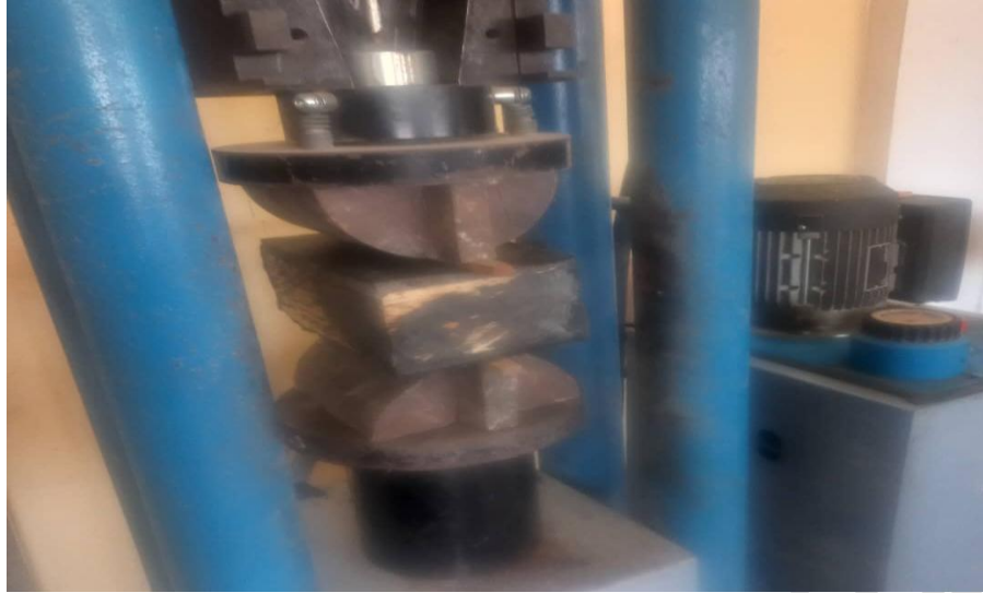
Fig. 4: Split tensile test of plastic brick
