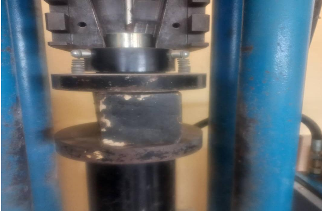
Fig. 3: Compressive strength test of plastic brick
