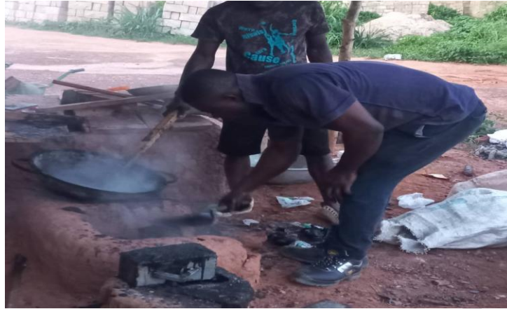
Fig. 2: Moulding of plastic bricks in the laboratory
