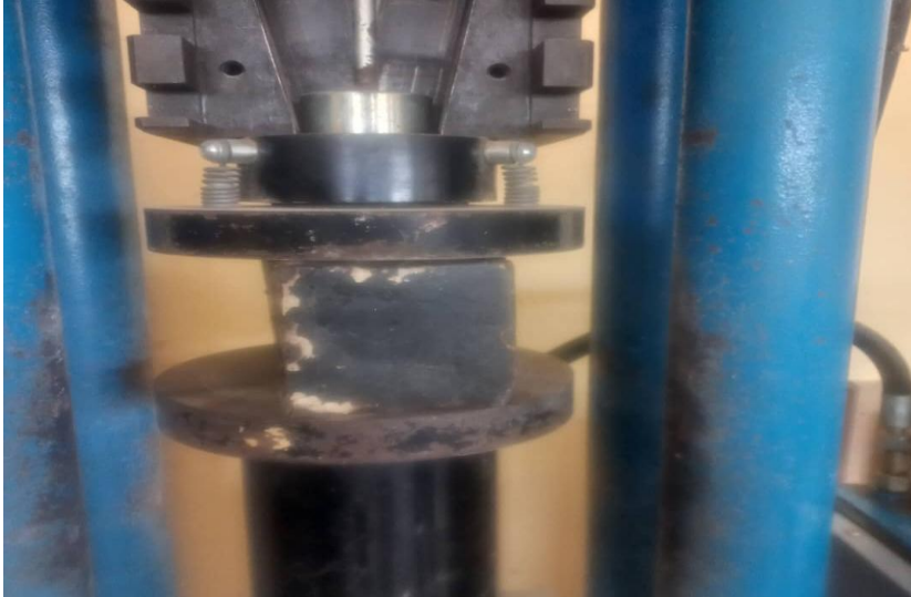
Fig. 3: Compressive strength test of plastic brick
