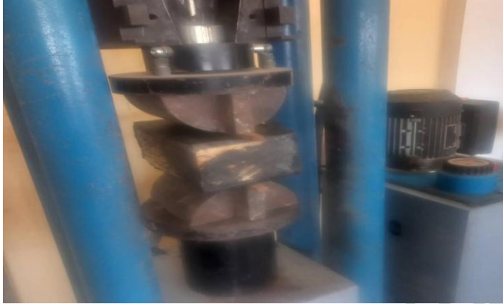
Fig. 4: Split tensile test of plastic brick
