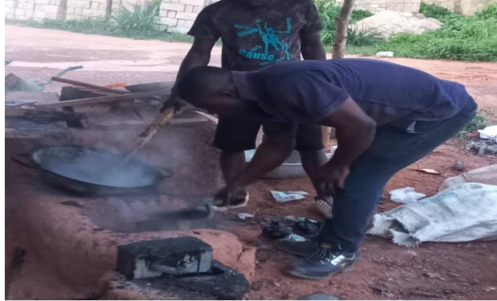
Fig. 2: Moulding of plastic bricks in the laboratory
