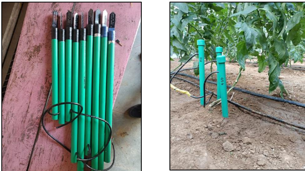
Fig. 3 Installation of the capacitive soil moisture sensors at different depths
