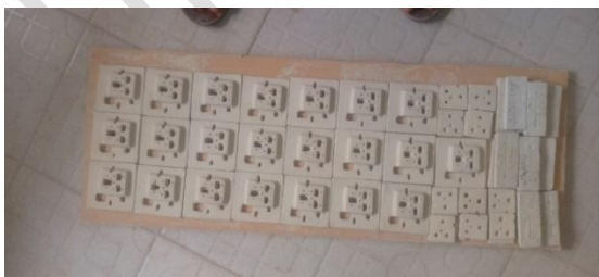
Fig 10: Fired Samples of the Socket
