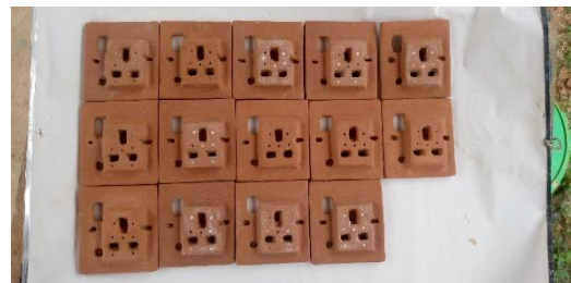
Fig11: Fired Samples of the Socket
