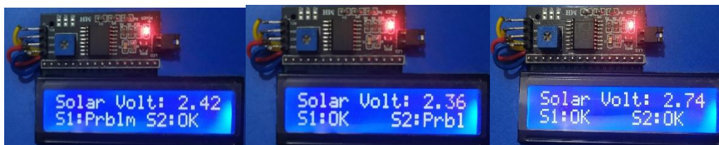
Fig.10. Generated voltage and branch connection statuses on the LCD screen.
