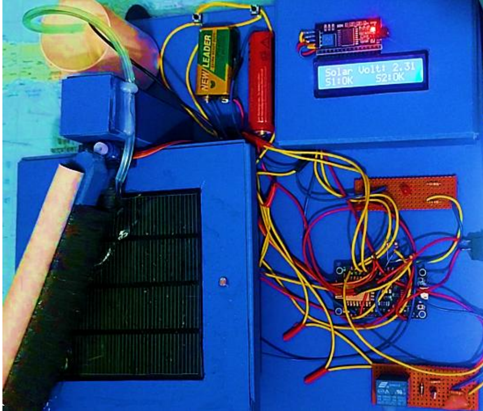
Fig. 11. Water reservoir with the pump and servo motors with cleaning brush.
