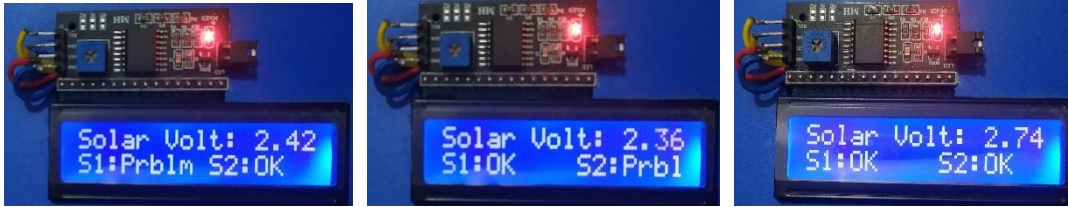
Fig. 9. Generated voltage and branch connection statuses on the LCD screen.
