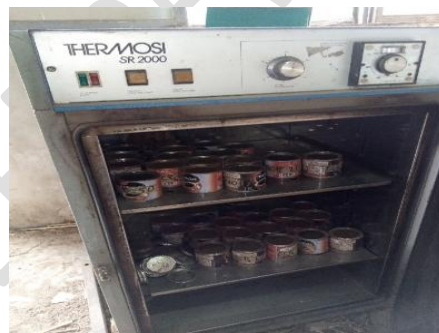
1-b : Oven drying of samples
