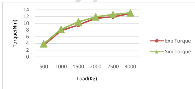
Fig 2: Variation of engine torque with load increase for D95 fuel sample
