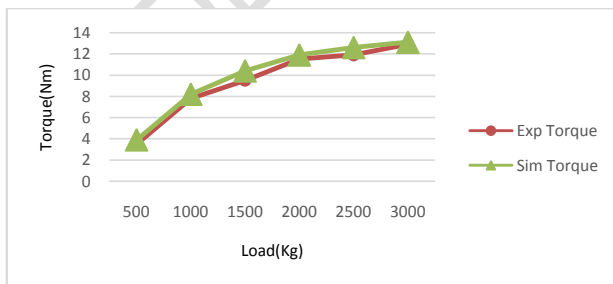
Fig 2: Variation of engine torque with load increase for D95 fuel sample
