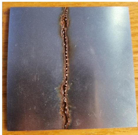
Fig.4 Stainless steel plate welding through
