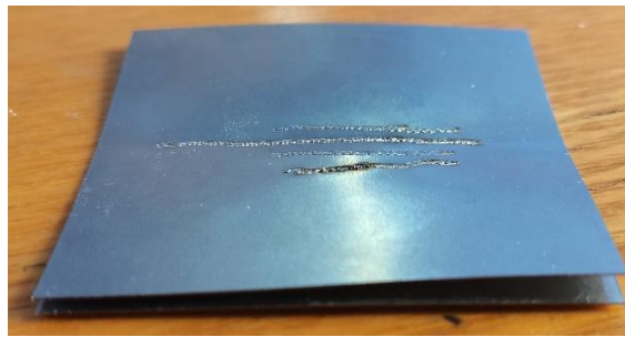
Fig.3 Laser welding of stainless steel plates without using fixtures
