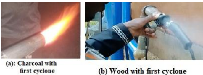
Figure 9 : Syngas combustion with first cyclone with charcoal and wood as combustible
