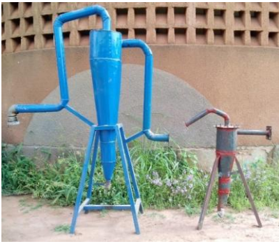
Figure 5 : Comparison of the two cyclones separators
