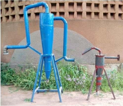
Figure 5 : Comparison of the two cyclones separators
