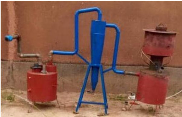
Figure 2 : Experimental setup with first and second cyclone
