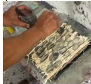
Fig. 8. Resin coating and production of bio-composite stage 3
