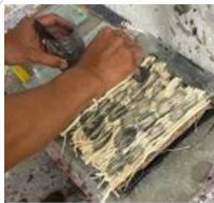
Fig. 8 Resin coating and production of bio-composite stage 3
