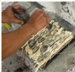
Fig. 8 Resin coating and production of bio-composite stage 3
