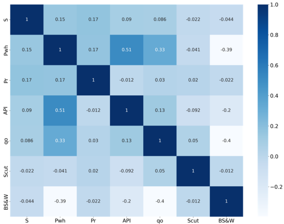
Figure 4: Correlation plot of the input variables with output - S_{cut}
