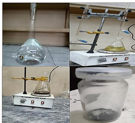
Fig. 6. Steps for the Synthesis of Bi-Mg Bimetallic Nanoparticles
