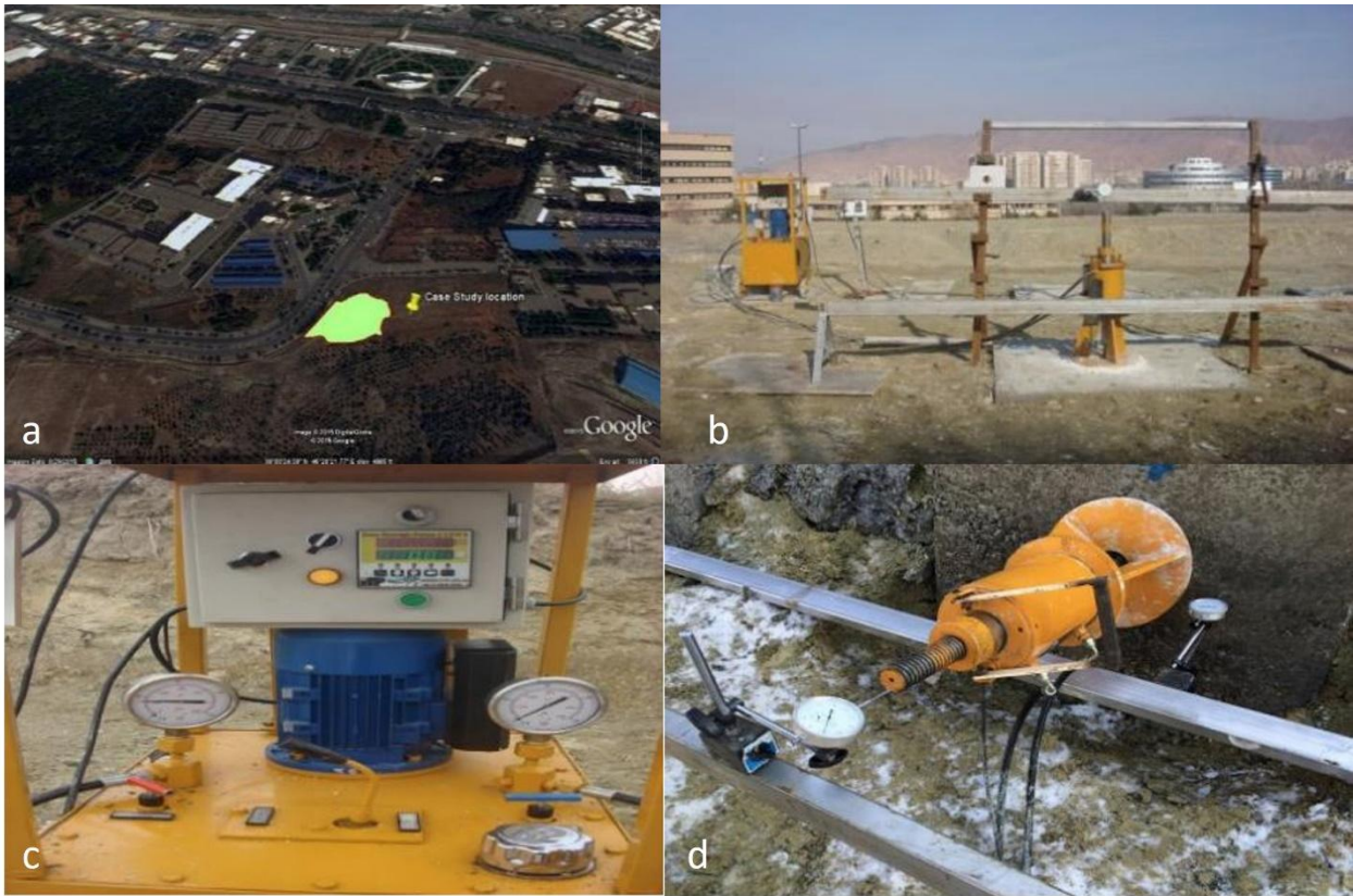
Figure 1. Aerial image of the study site along with the tension-compression jack and its peripherals. (a) areal images of the study site. (b) The jack system and its accessories installed at the study site. (c) Data logging and pressure calibration device. (d) The interface connecting the jack to the anchor and installation of measurement gauges. Axial displacement of the anchor and the concrete pad settlement.
